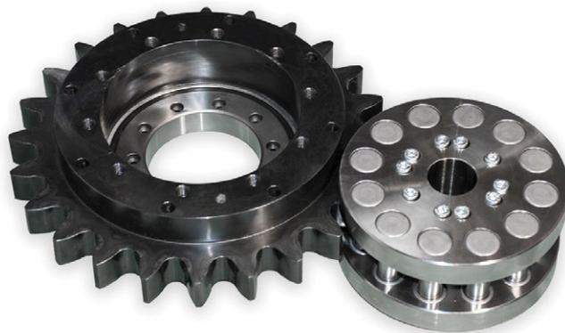
**Nexen's Rotary Indexer System is based on the company's innovative Roller Pinion System (RPS) for linear motion. To create a Rotary Indexer, the linear rack becomes a circular gear. Instead of moving a linear rack side to side, the pinion rotates the gear. The pinion gear is equipped with bearing-supported rollers that engage a unique tooth profile in the gear, providing smooth rolling friction instead of sliding friction.**
